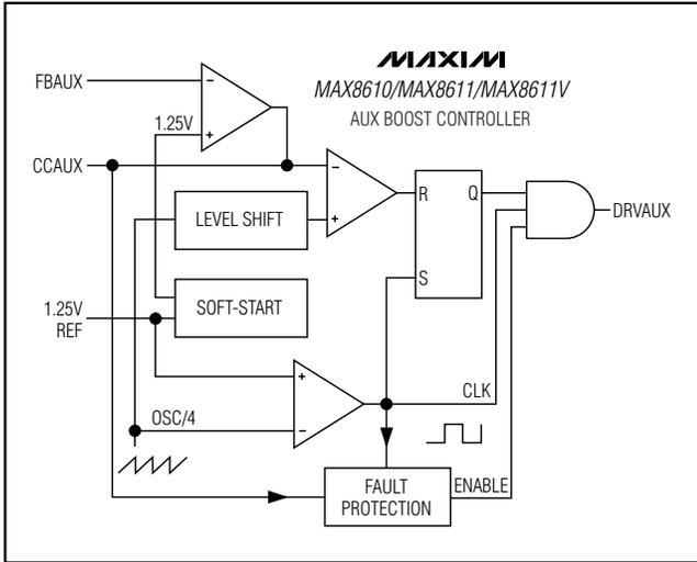
Figure 4. AUX Boost-Controller Block Diagram
