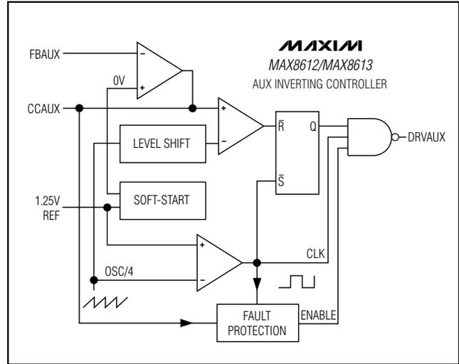
Figure 5. AUX Inverter-Controller Block Diagram
