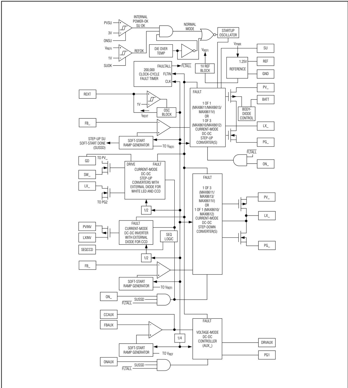
Figure 3. MAX8611 Functional Diagram
