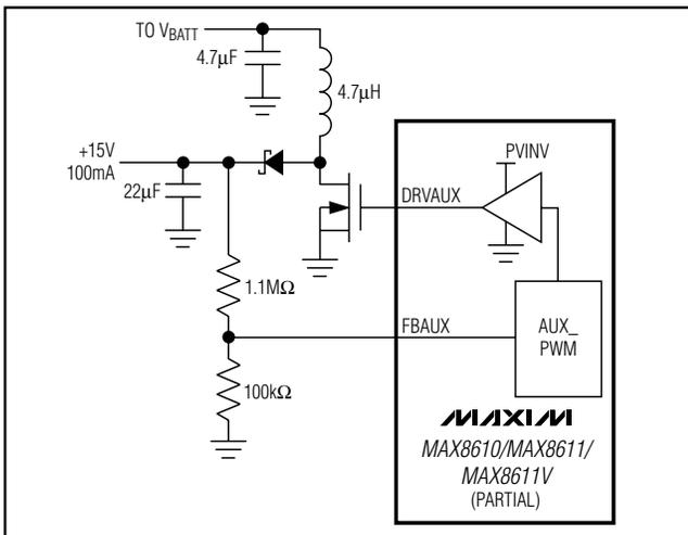
Figure 8. Typical Application for the AUX Boost Controller on the MAX8610/MAX8611/MAX8611V
