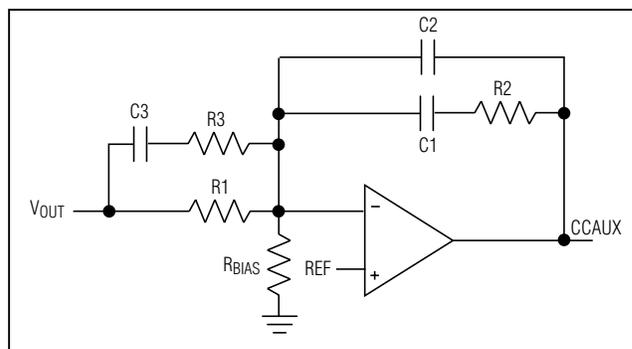
Figure 7. Type 3 Error-Amplifier Circuit
