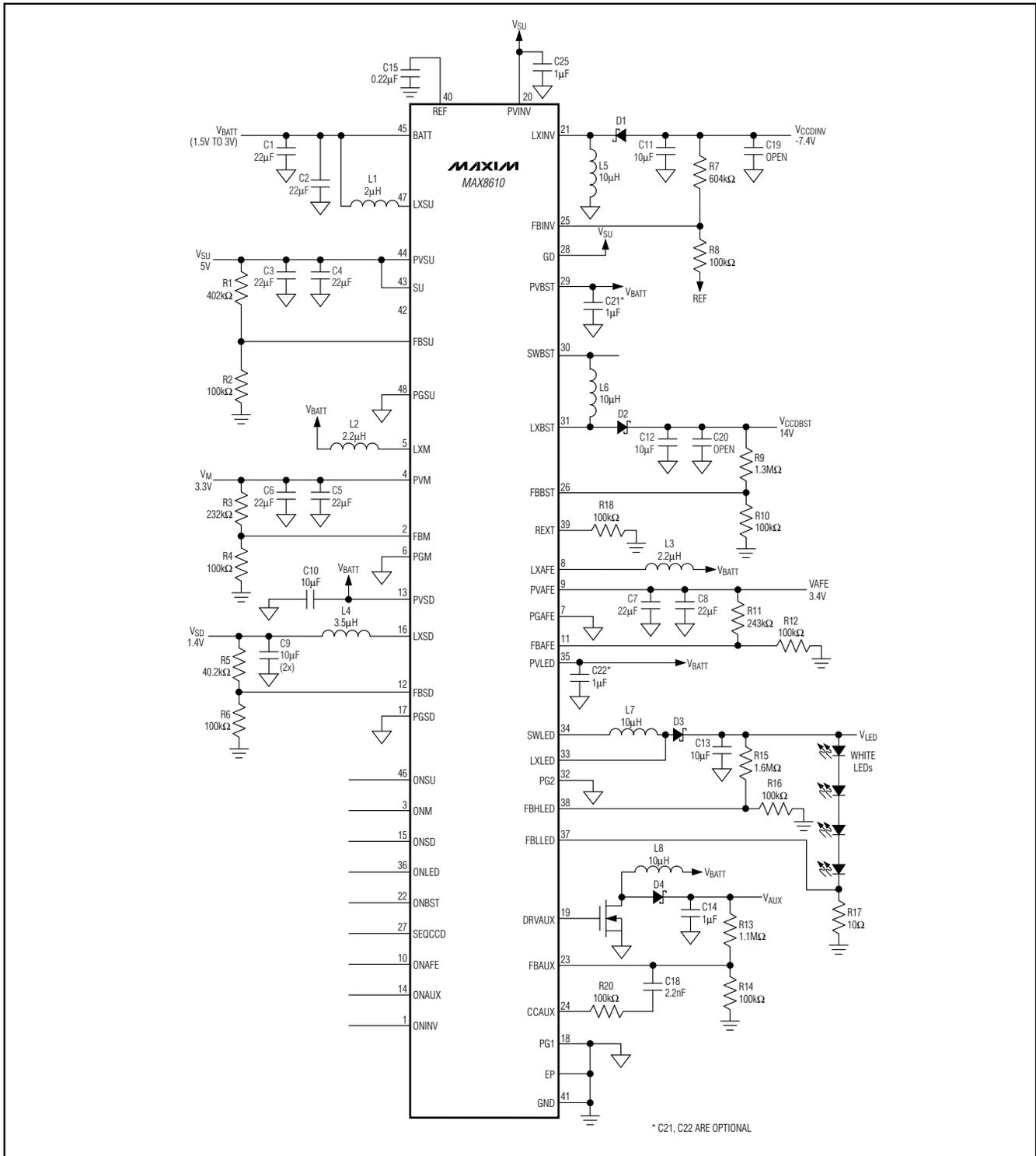
Figure 1. MAX8610 (2 AA Input) Typical Application Circuit. The MAIN and AFE outputs operate as step-up converters.
