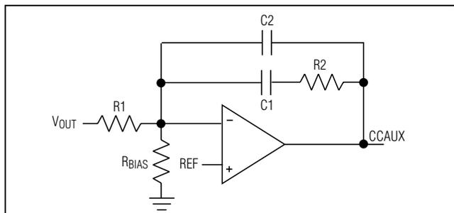
Figure 6. Type 2 Compensation Circuit
