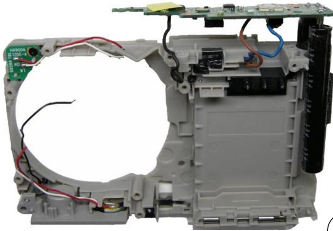
(The work will be easier by taping temporarily the CONDENSER to the INNER HOLDER .)
