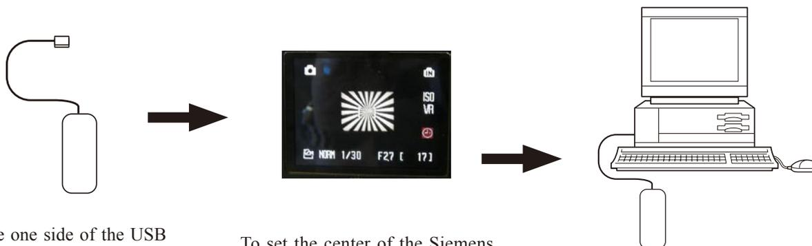
Connect the one side of the USB cable (UC-E10) △ (Addition) to the camera (without connecting the other side to the PC).
