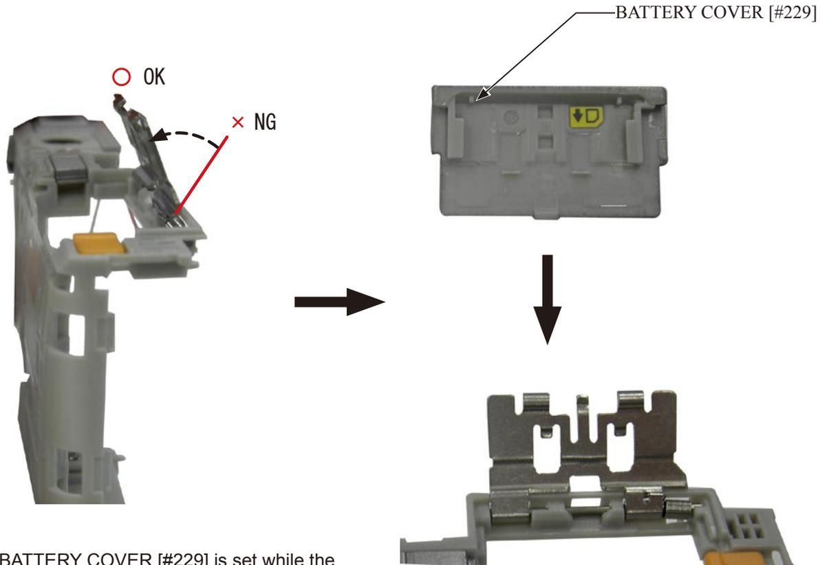
Note: If the BATTERY COVER [#229] is set while the metal plate is at the full open position, the INNER HOLDER will be damaged. Set the BATTERY COVER [#229] while the metal plate is closed a little as shown in the photo.
