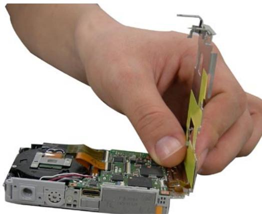
Note: Because the FPC is short in length, set it while holding the LCD HOLDER.
