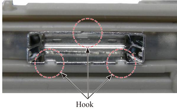
Be careful that the hook of the reflector on the FLASH LAMP can be easily bent.
