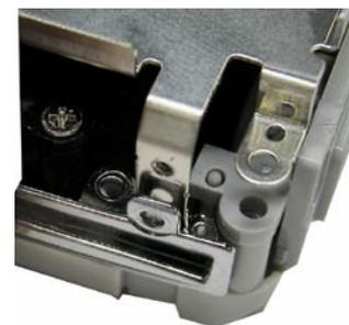
The lower part at the lens side can be removed easily by releasing DECORATION RING.
